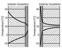
2 The temperature profile shows that the exterior wall remains colder in the winter through interior insulation
