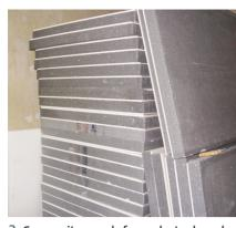
3 Composite panels from plaster board (white) and insulating boards of Neopor (silver-grey)
